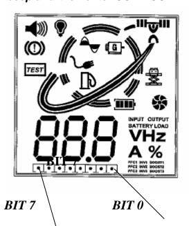
Note that on the display panel, you will see a single row, 8 BIT column located at the bottom of the display. The most right bit is function "BIT 0", the far left is status "BIT 7". Note that there is an illuminated dot "." in BIT 0 when the unit is in CONFIGURATION MODE.
